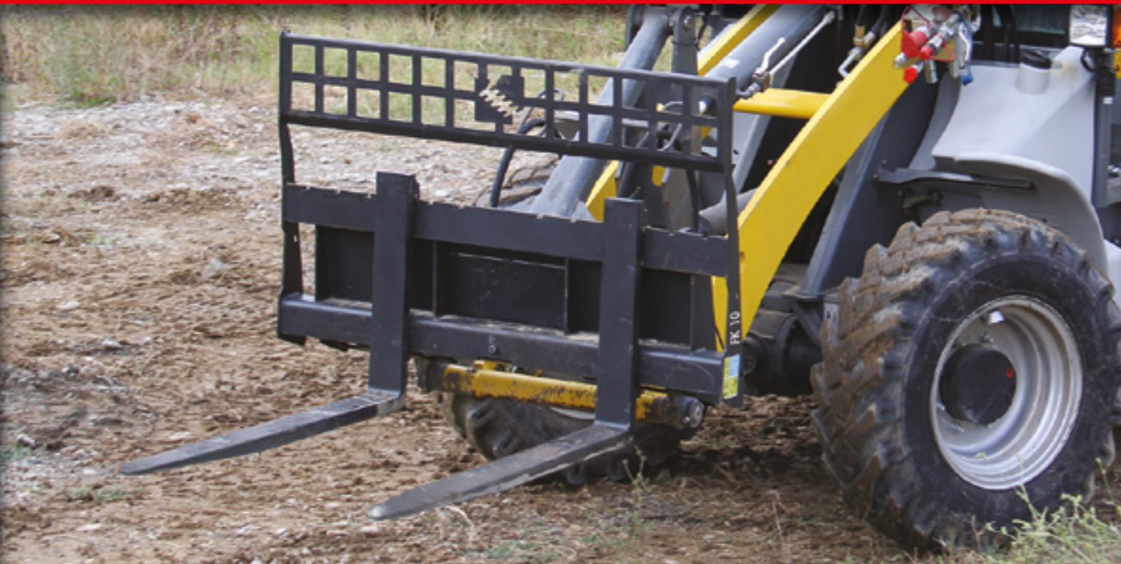
FRONT PALLET FORK FOR SKID, WHEEL, TELESCOPIC AND BACKHOE LOADERS. EQUIPPED WITH A SAFETY SYSTEM TO AVOID THE TILTING OF LOADS DURING ITS USE.
