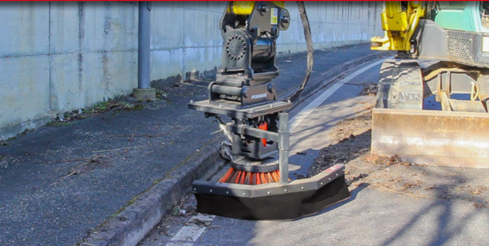
IT DEEPLY CLEANS CURBS, SIDEWALKS, BANKS AND ASPHALTED AREAS AND REMOVES WEEDS.
